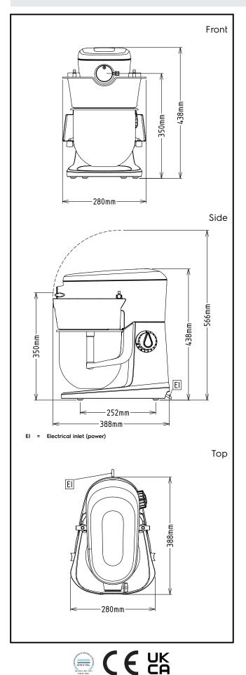
Electric Supply voltage: 200-240 V/1N ph/50/60 Hz **Total Watts:** 0.5 kW Capacity: Performance (up to):
